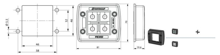
Torque for the frame's mounting screw: 2.5 – 3 Nm
